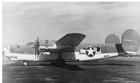
USAAF Anti-Submarine Liberator. The retracted radar dome is barely visible behind the open bomb bay. (Credit: USAF-USAAF)
