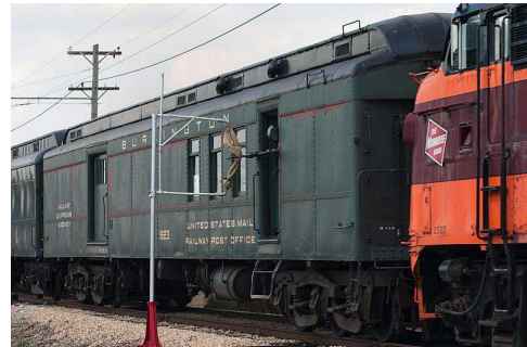
The exact moment in which the catcher pouch is snatched from the crane. (Credit: M. Michael Miley)
