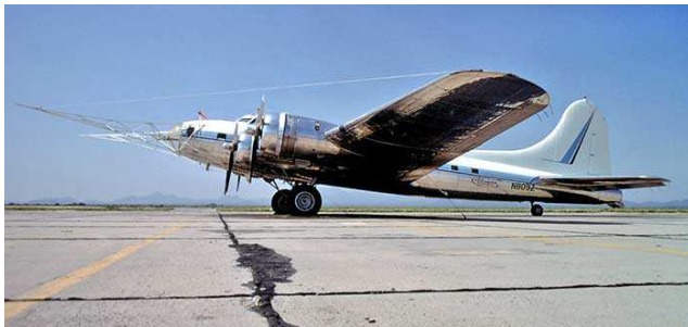
Note the wire protectors to prevent the lifting cable from being dragged into a propeller. (Credit: Neil Aird)
