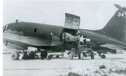
The Curtiss C-46 Commando could carry twice the payload of a C-47.
