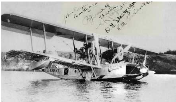
The PN-9 after rescue. Note how the fabric has been peeled from the lower starboard wing to fashion a sail. (Credit: Library of Congress)
